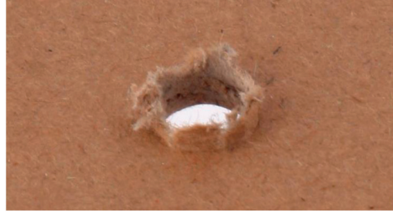
rough side of a punched hole
