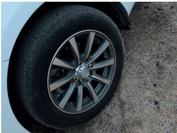
Figure 13: A rubber tyre is a shell structure.
