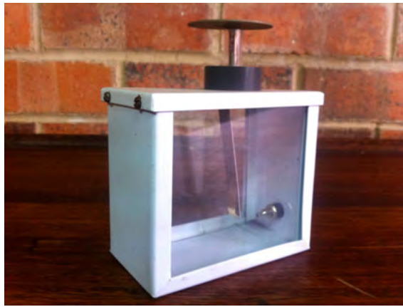
An electrostatic induction demonstrator used in a laboratory.
