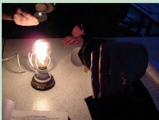
Viewing a light source through a pinhole camera with different lenses.
