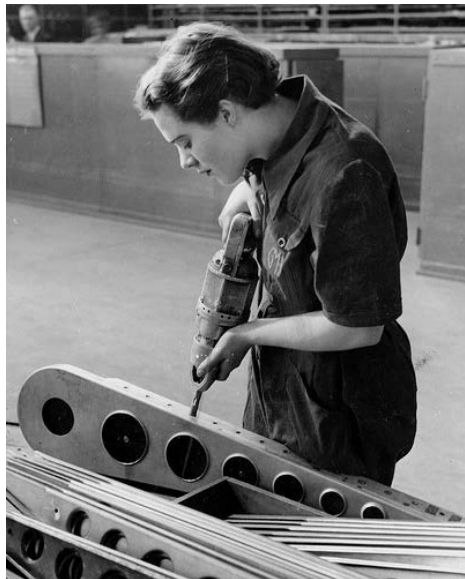
A lady using an electric drill to make a hole in an aeroplane part.
